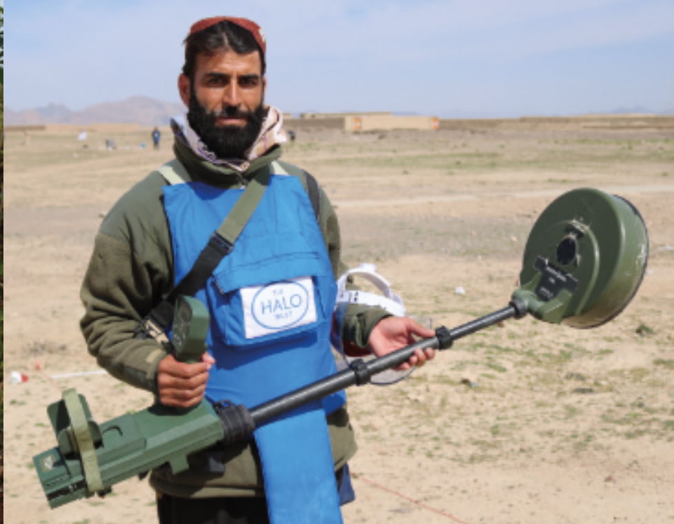
Primary search method in Afghanistan for manual IED clearance - Vallon VR1 Wirehound detector (GPR)
